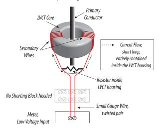
Additionally, since the current flow loop is much shorter (contained within the LVCT housing), burden capacity is no longer an issue. The internal resistor and the number of secondary windings can be selected to generate a high accuracy signal at all current ratings.
